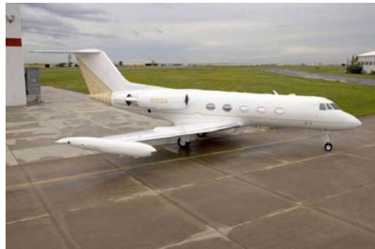
Figure 1: Fugro EarthData's GeoSAR. A purpose-built Gulfstream II business jet serves as the collection platform for X- and P-band IFSAR data.
